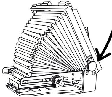
⑤ Screw front standard into desired base mount (see page 10 for guidance).
