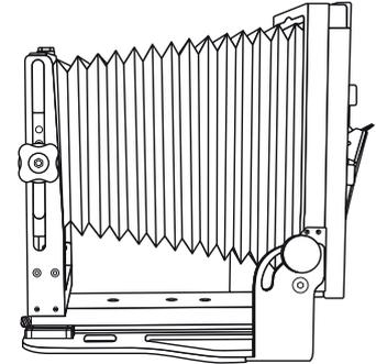
③ Tighten screws and lock rear standard at 90°.
