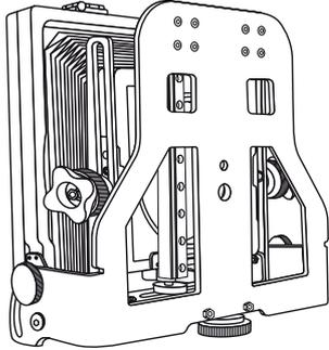
② Loosen rear standard screws and raise the rear while pulling front forwards.
